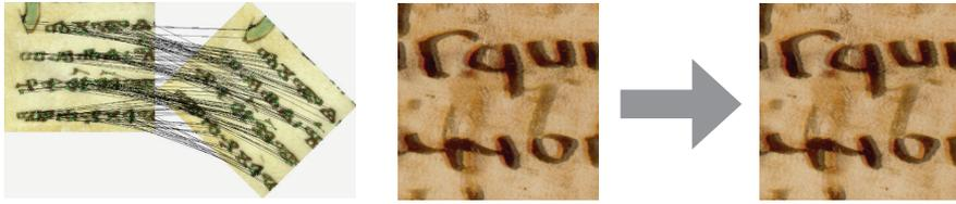
Fig. 2: Coarse Registration – Scale-Invariant Feature Transform (SIFT) based approach (left). Fine Registration – Modality Independent Neighbourhood Descriptor (MIND) approach from medical image processing (right).
