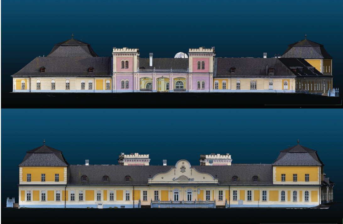
Figure 50. Žehra, Hodkovce (Slovakia). Manor house (18-19 th century), exterior. lBM in combination with TLS. Ortho-views of the facades.
