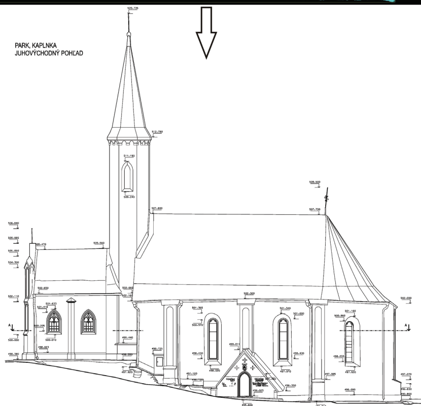
Figure 59. Žehra, Hodkovce (Slovakia). Neo-Gothic church (19 th century), exterior. Example of 2D vectorisation of ortho-rectified south facade.
