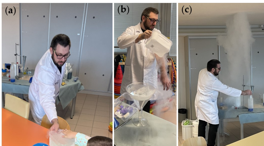
Figure 2. Demonstration experiments with liquid nitrogen: (a) cold vapours of liquid nitrogen can already be felt with the hand near the container, (b) Leidenfrost effect of liquid nitrogen on the skin and (c) gas leakage through the capillary: nitrogen fountain (Photo: Alenka Klun with permission of the University Medical Centre Ljubljana).
