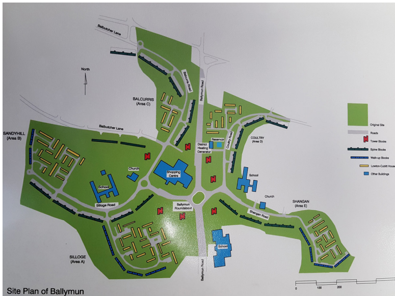
Figure 11: Site plan of Ballymun. Red colour indicates the position of seven tower blocks, dark green colour indicates the position of lines of spine blocks, dark blue refers to the position of walk-up blocks, yellow refers to Lowton-Cubitt houses and flats, and light blue refers to other buildings (schools, churches, shopping centre, boiler house). Source unknown, year unknown. Courtesy of the Ballymun Community Archive, Ballymun Library.
