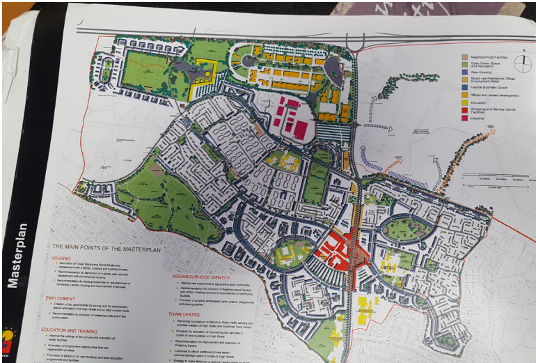
Figure 17: One of the pages of BRL Masterplan for the Ballymun regeneration. The photo shows a plan of New Ballymun, with violet colour referring to new housing, orange to office space and red to shopping facilities. Main points of the Masterplan are summarised on the left bottom side. (BRL Masterplan 1998: 1). Courtesy of Ballymun Community Archive, Ballymun Library.
