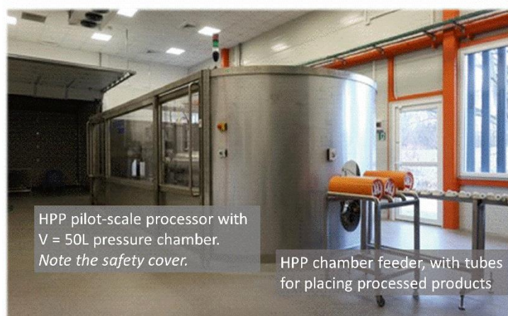
Figure 6. HPP pilot processor with V = 50\text{L} pressure chamber for the industrial-scale test, finalization of implementation protocol, and market experiments. X-Press Matter Lab, IHPP PAS (X-PressMatter, 2024).
