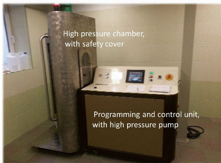
Figure 5. HPP lab scale processor with V = 1\text{L} pressure chamber, for basic research and preliminary establishing of implementation protocols for “HPP foods”. X-PressMatter Lab, IHPP PAS (X-PressMatter, 2025).
