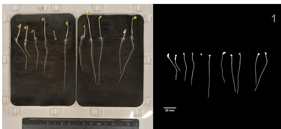
Figure 1. Visual example of germination test (left) and evaluation of roots length with ImageJ app (right)
