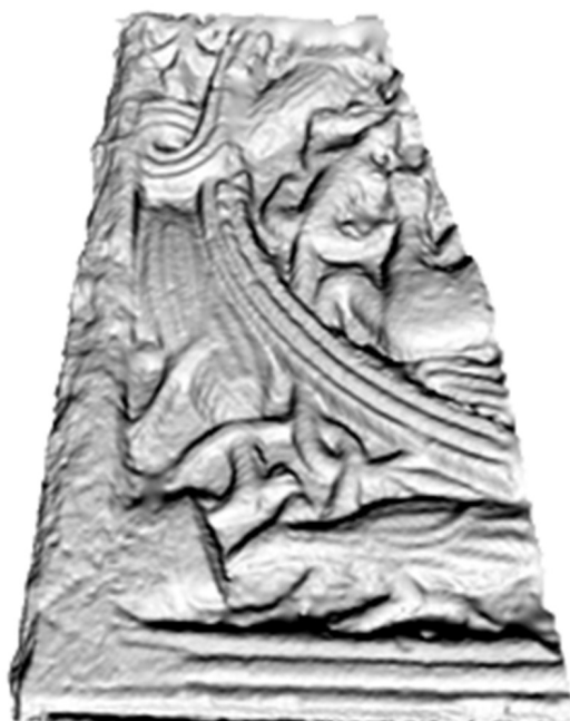
Figure 36. Meshlab (mesh), Model 2 created by Visual SFM (dense point cloud) and Meshlab (mesh).
