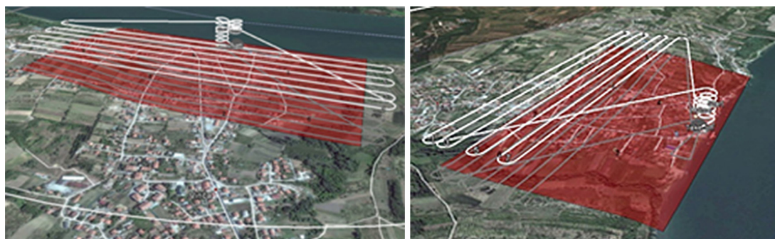
Figure 13. Flight plan and trajectory of the drone used to acquire digital elevation model of Vinča Belo Brdo.
