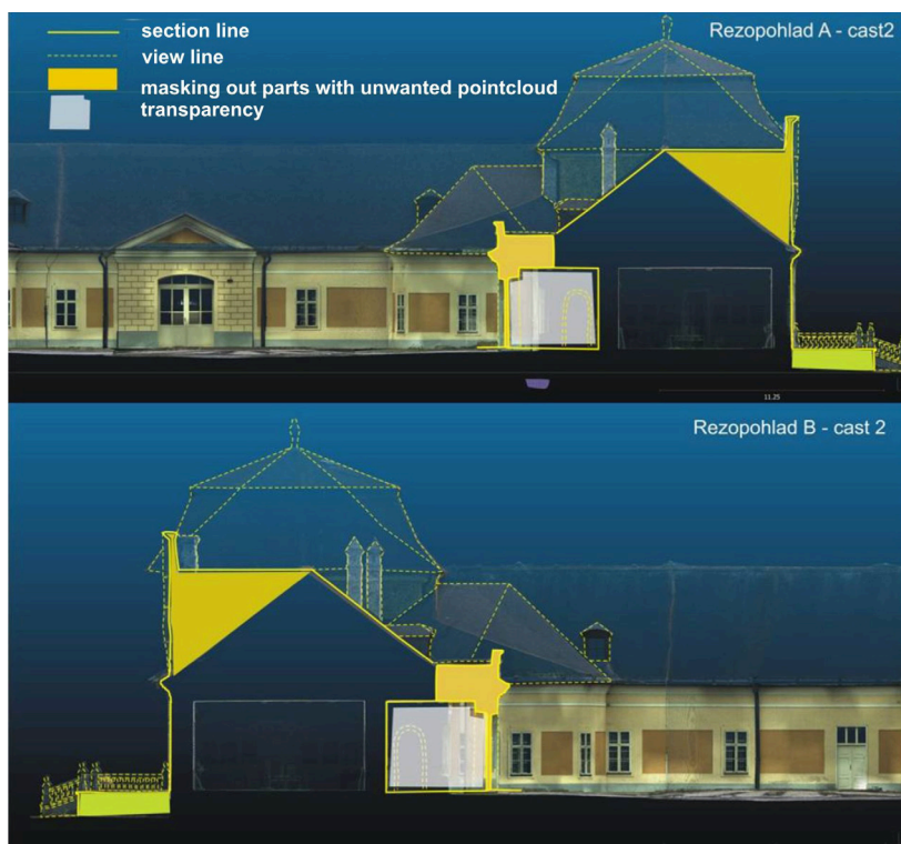
Figure 58. Example of unwanted transparency of the point cloud in the generation of a cross-sectional view.
