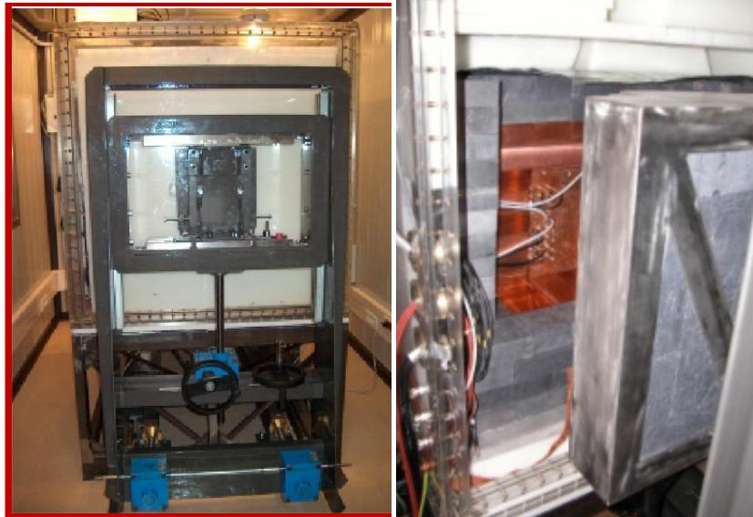
Fig. 6.7: Photos of the DAMA/R&D set-up: *Left* - the multi-component closed shield, which surrounded the inner OFHC Copper box housing the detector(s) in HP-N<sub>2</sub> atmosphere; *Right* - partially open shield, showing the inner OFHC Copper box.
