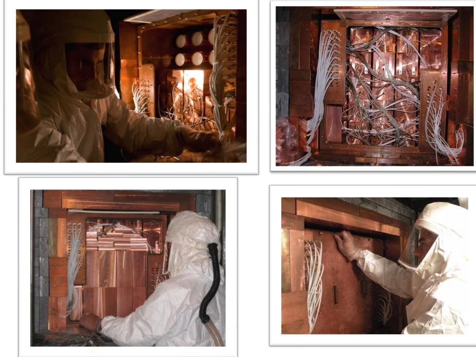
Fig. 6.3: Photos during installation in HP-N<sub>2</sub> atmosphere of the NaI(Tl) detectors in the inner high purity copper box which is surrounded by the multi-tons multi-materials passive shield.
